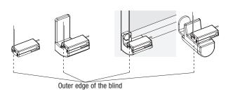
Recommendation: DIN 7982 Ø 3.9 x 13 mm (for wooden and synthetic frames)
