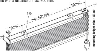
Attention: It is recommended to mount the clip with the flap forward (into the room). The clip can **only** be mounted with the flap toward the window or the pane respectively, in case the distance to the rail is min. 7 mm.
